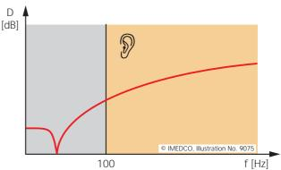
Where the mass of the floor is particularly high, it can only be excited to a small degree by MRI vibration. Single elastic supports are usually all that are needed to optimally decouple the MRI equipment from the building structure and provide adequate soundproofing in the audible range (100 Hz to 20,000 Hz).
