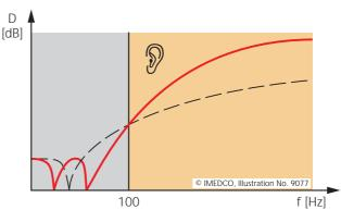
What is used for the additional mass, its dimensions and the type of support depend on the building structure and the make and model of MRI equipment. An elastic system having two degrees of freedom achieves better noise reduction.
