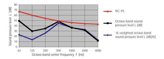
The **octave band sound pressure level** is the true NON-WEIGHTED energy sound pressure level of a typical MRI system measured in the control room (incl. RF door and RF window).
