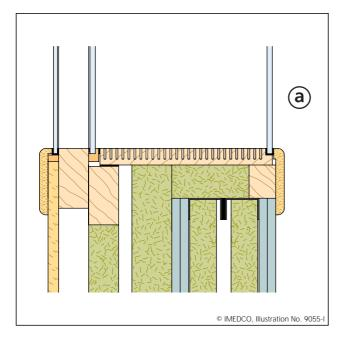
Thin panes of glass suppress high frequency sound waves very well and thick ones suppress low frequencies. An effective soundproof window therefore includes thin and thick panes of glass.
